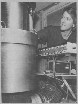
MARY YOUNG (7531) checks the rotary joint assembly atop the centrifuge. The rotary joint, which Mary designed, allows wiring and cooling air to reach the shaker even when the centrifuge is spinning.
